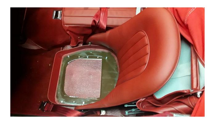
The seat bases are painted brown, as are the inside of the instrument panel, transmission tunnel, glove shelf and other metal parts, as I believe they were from the factory.
