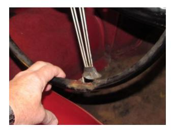
As you can see, someone actually tried to use a wood screw to mend the break in the wheel rim. This photo shows how we ground the plastic away, so we could weld the spokes back
