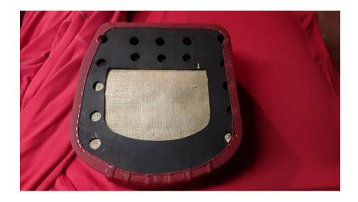
Lynn points out that the burlap material is not correct as the foam cushion was exposed as it came from the factory. Also, the factory used tacks, not staples, to secure the leather to the base. Here is a photo of Lynn's seat.
