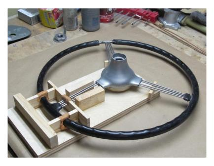
We poured West System G-Flex epoxy, mixed with micro-balloon filler and black pigment, into the mold. The result was then sanded to match the contours.
