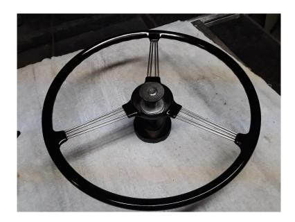
This is the finished result, after having been painted black, with a single stage urethane automotive paint. The fitting in the hub was to support the wheel during painting. It is satisfying to have saved the original wheel.
