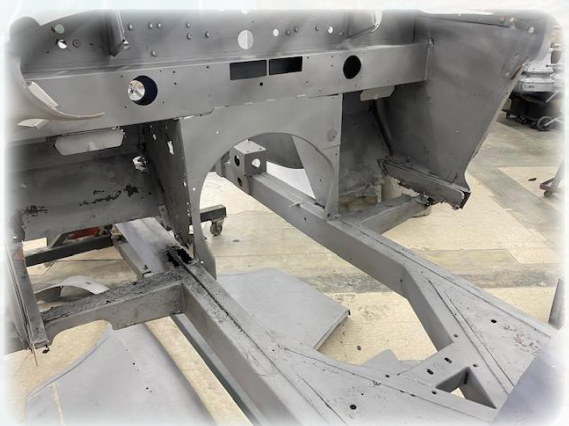
Figure 3: chassis sandblasting revealing the extensive metal restoration required.
