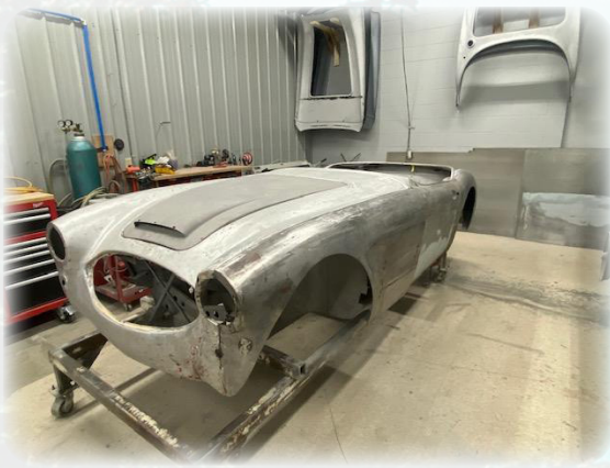
Figure 4: after chassis is restored the body panels are fitted to insure proper alignment.
