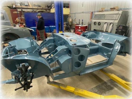
Figure 5: restored chassis primed and painted.
