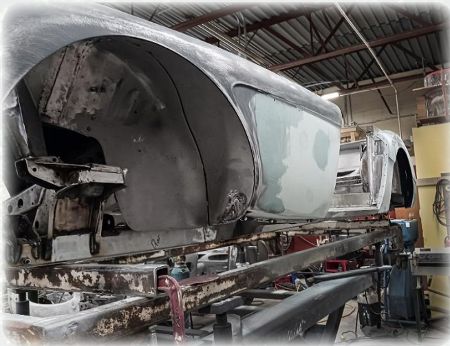
A repeated process of skim coat, sand, and reprimed till perfect
