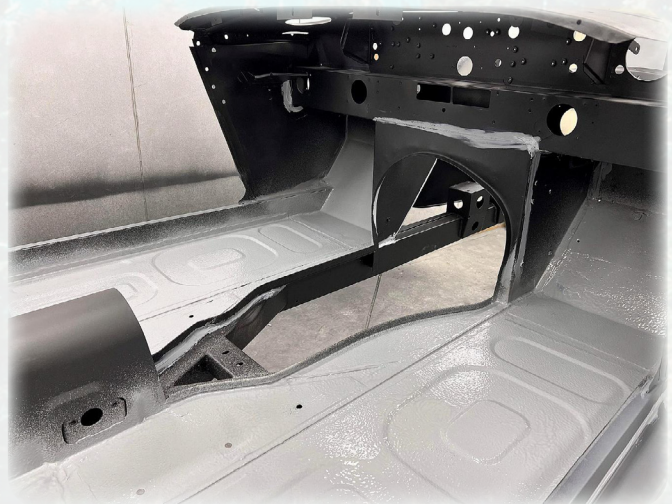
Chassis primed with floors painted with Stone Guard.
