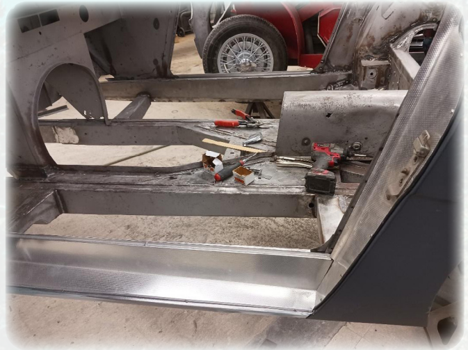
New rockers, pillars, and inner and outer sills.
