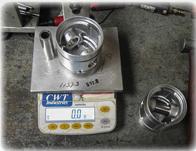
New balanced pistons and connecting rods
