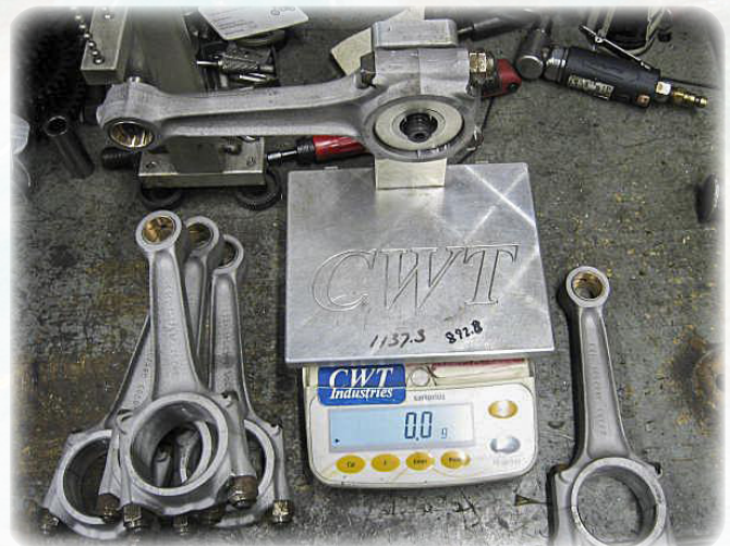
New balanced pistons and connecting rods
