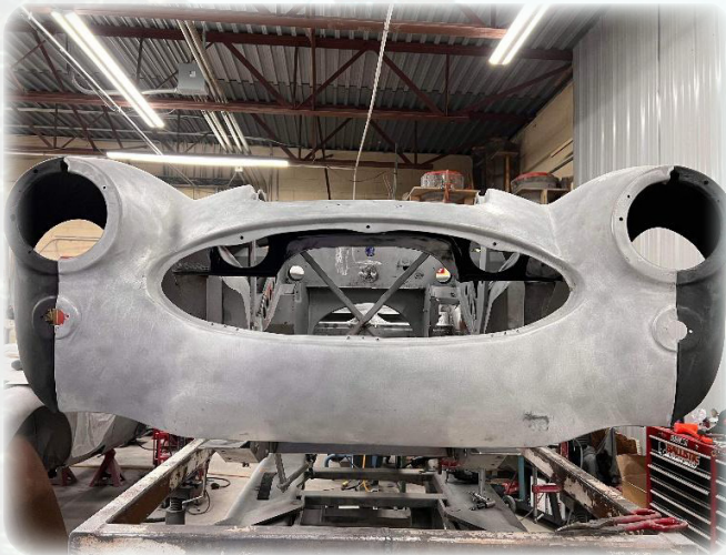
Primed Body Panels being fitted
