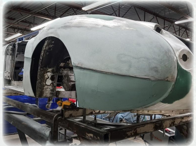
A repeated process of skim coat, sand, and reprimed till perfect
