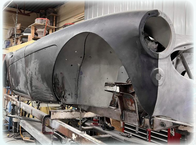
Primed Body Panels being fitted
