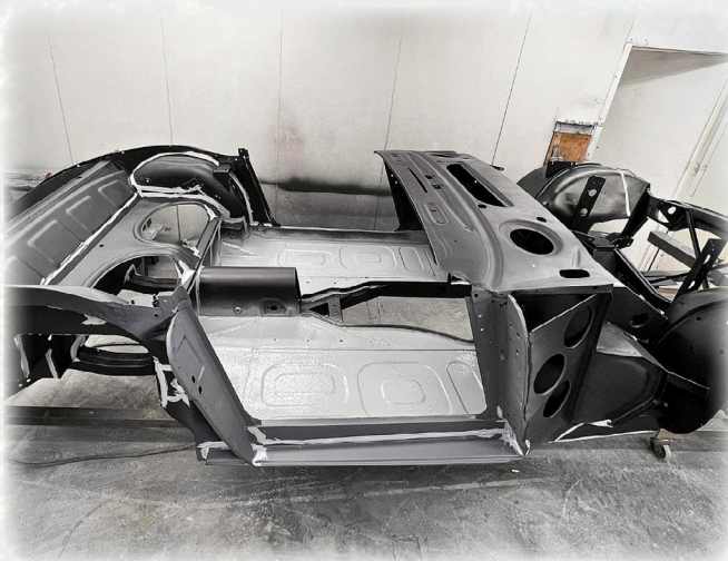
Chassis primed with floors painted with Stone Guard.
